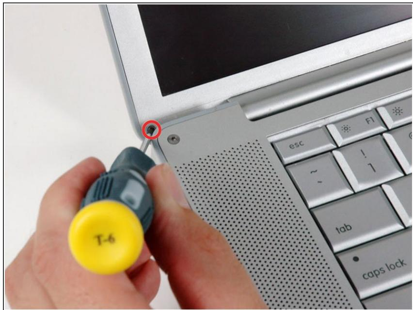
**i** The following procedure allows the changing of the rear display bezel without removing the display assembly from the computer. Do not attempt to rotate the display back farther than the hinges allow or your computer may be damaged.
